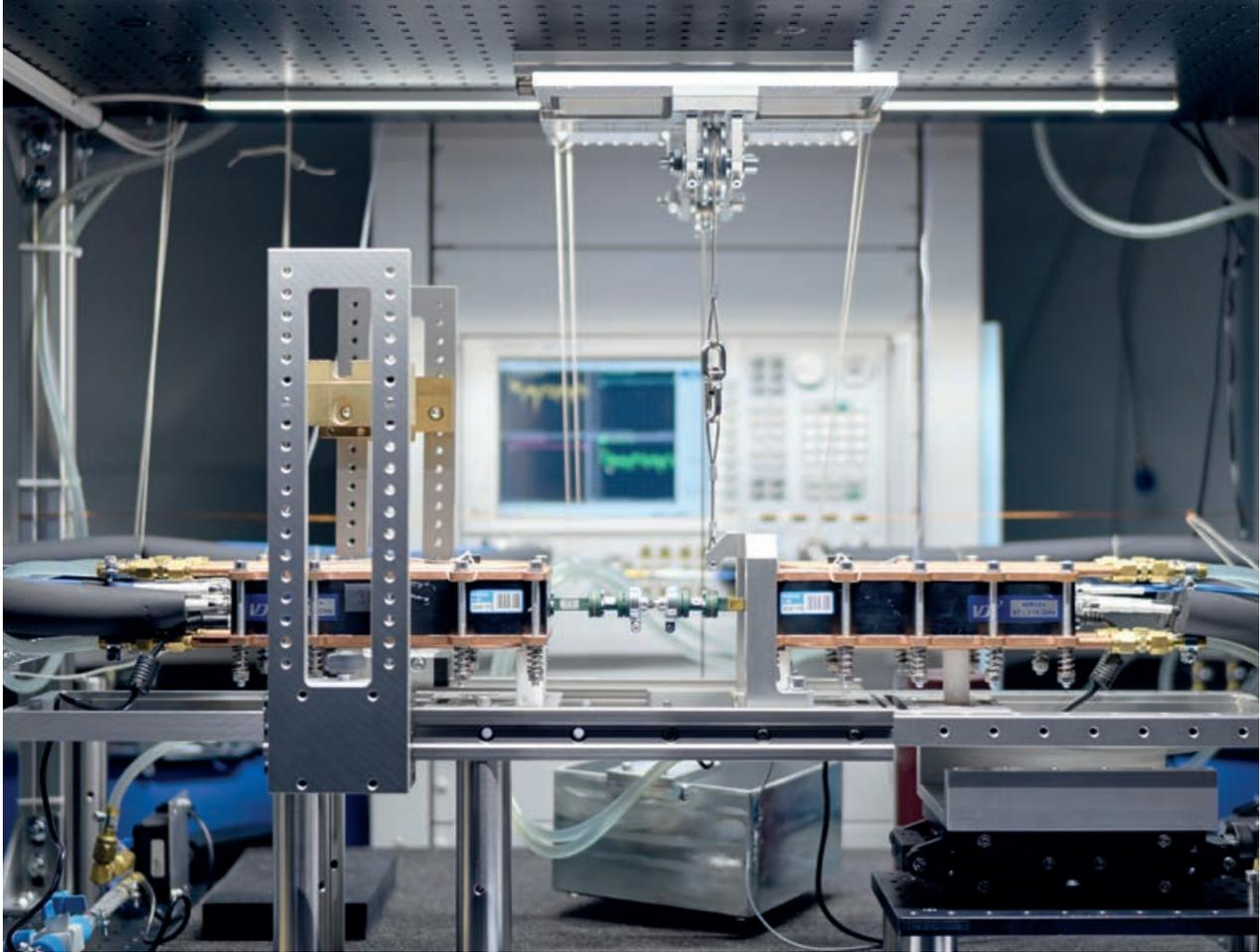
4: Measurement setup for the 1.0 mm measurements with the two extender heads in the front (the two black boxes clamped between copper plates). Unique features of the setup are a free floating suspension system and a water cooling system for temperature control.
