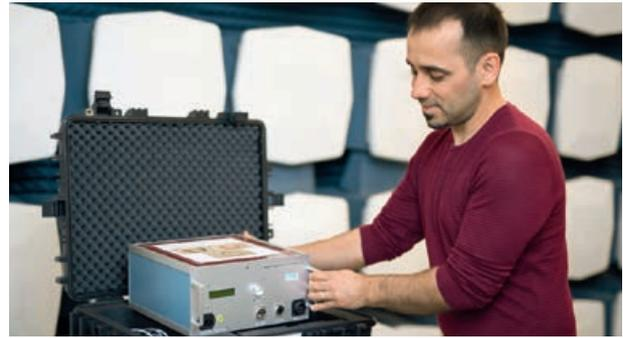
4: Device for validating conducted immunity tests in accordance with IEC 61000-4-6.
