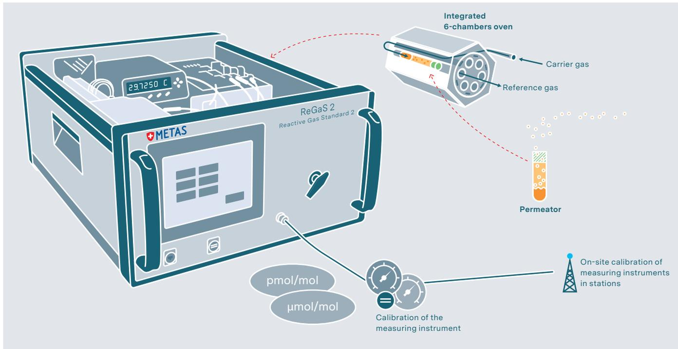
ReGaS generates reference gas mixtures based on permeation, allowing for on-site calibration anywhere.
