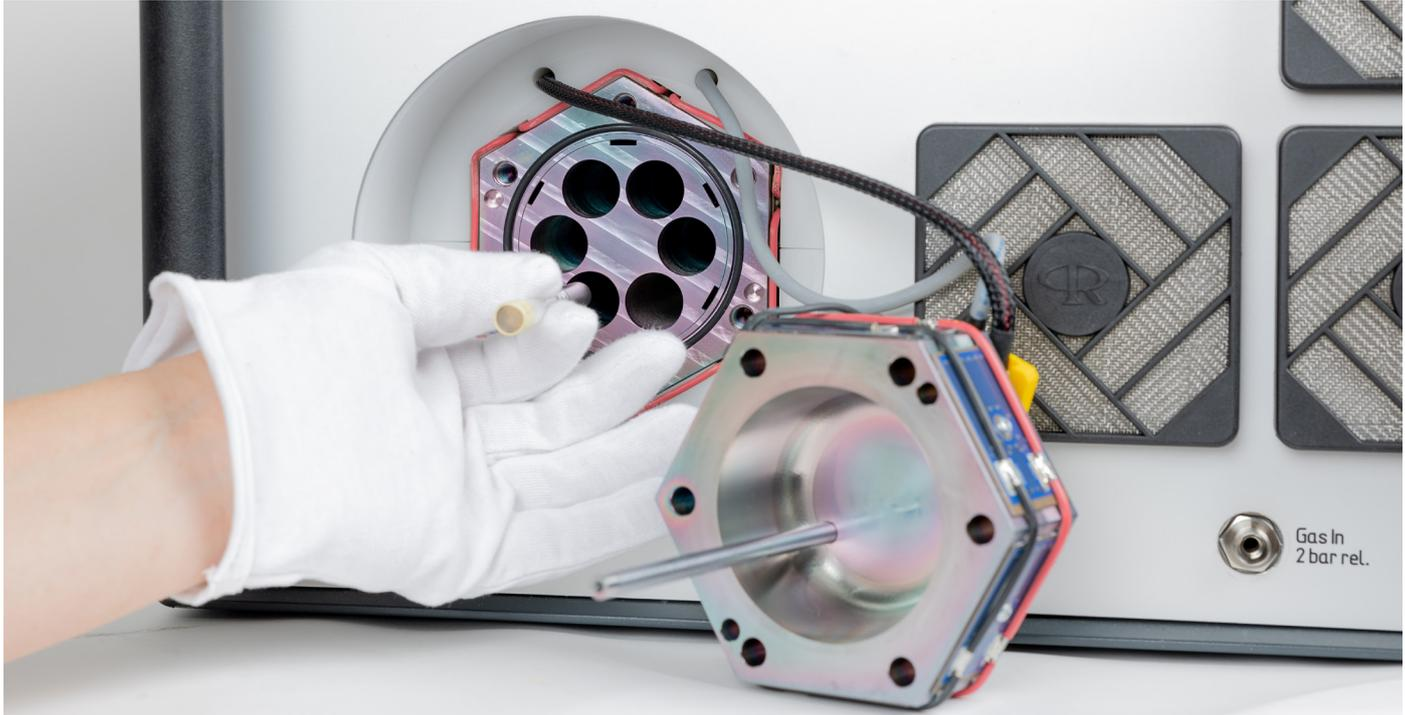
A permeator is being installed in the oven of ReGaS.
