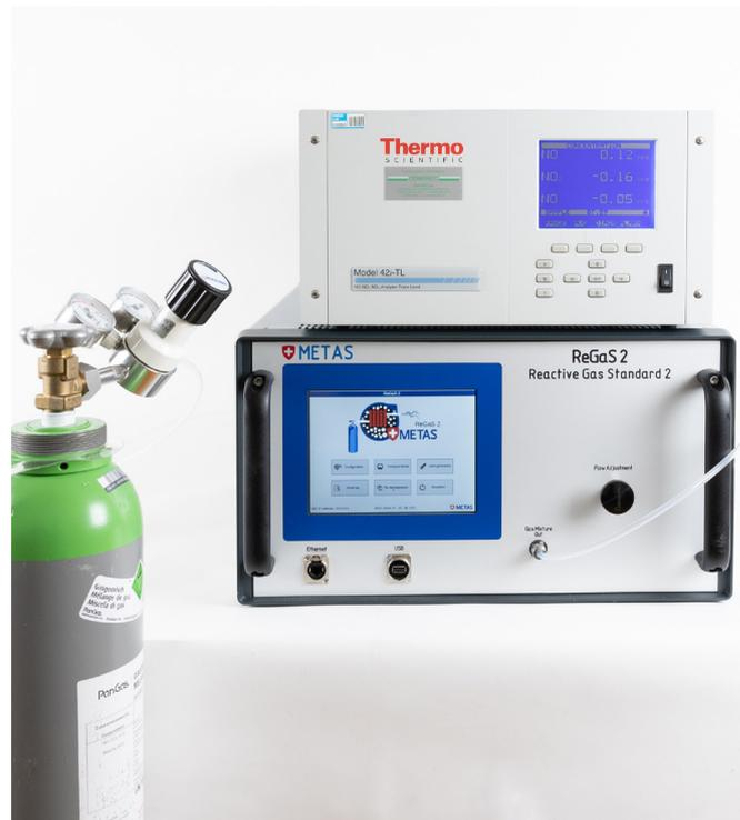
Calibration of an  $\text{NO}_2$  measurement device in the field using high-precision reference gas mixtures generated by ReGaS.
