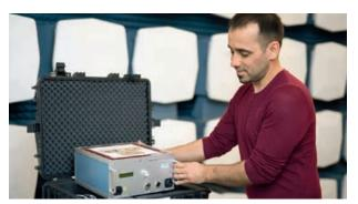
4: Device for validating conducted immunity tests in accordance with IEC 61000-4-6.
