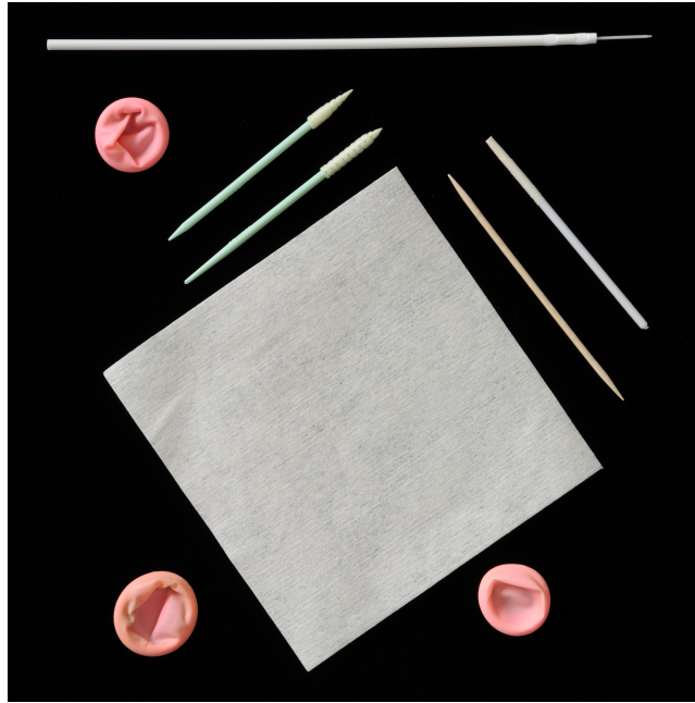
Figure 12: These are accessories for cleaning connectors. In the center one can see a lint free cloth. On the right hand side of the cloth one can see a wooden toothpick and a with lint free cloth wrapped stick. On the left hand side of the cloth one can see plastic picks for cleaning female center conductors of N-Type, 3.5 mm, and 2.92 mm connectors. At the top border, one can see a plastic pick for cleaning the female center conductors of 2.4 mm and 1.85 mm connectors. In the corners one can see finger cots which are used for handling center conductors of beadless components.
