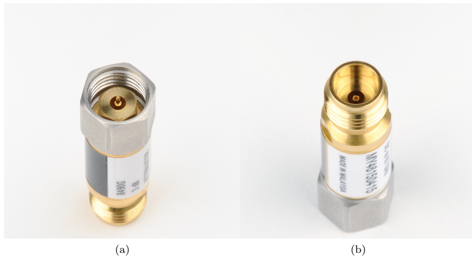
Figure 9: Male (a) and female (b) 1.85 mm connectors.
