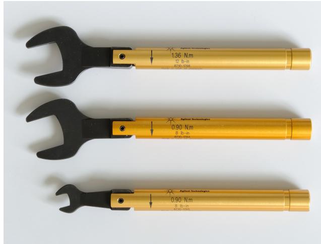
Figure 14: These are examples for torque wrenches. Note that there are different torques available for the same nut size.
